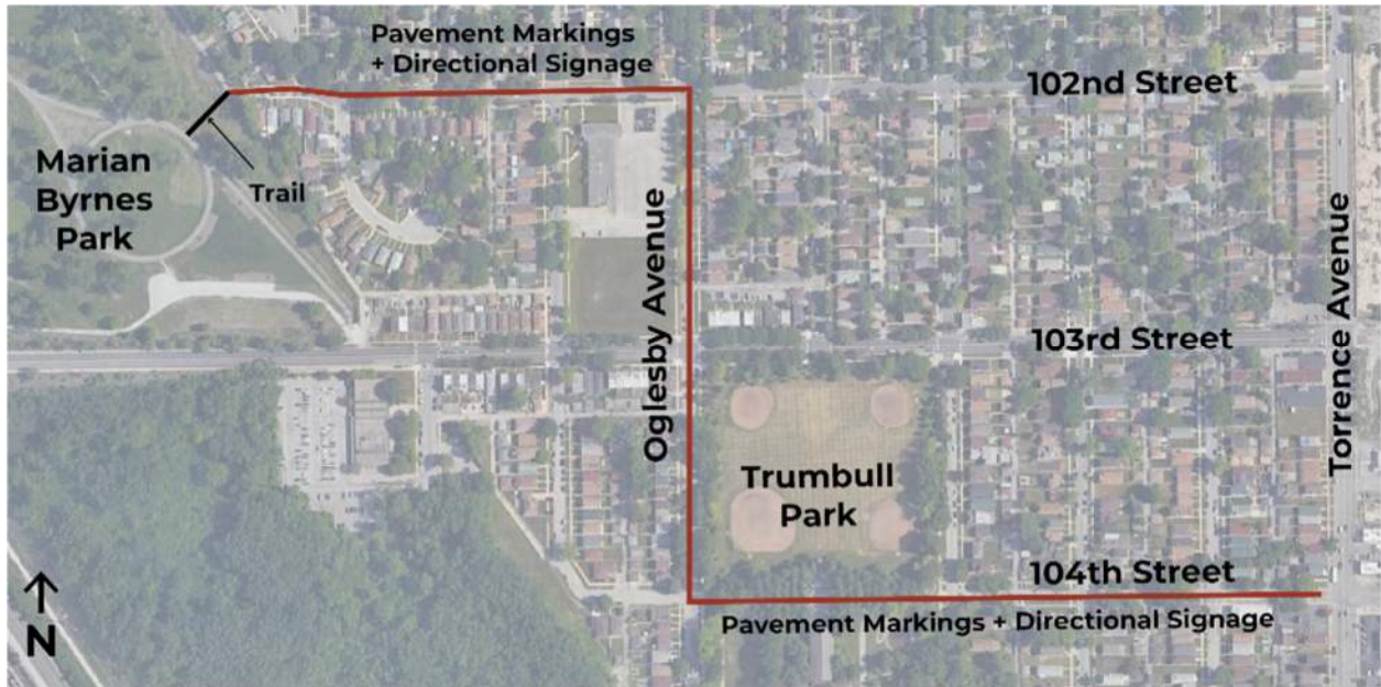
Figure 48: 102nd Street/Oglesby Avenue/104 th Street Improvements – Marian Byrnes Park to Torrence Avenue
